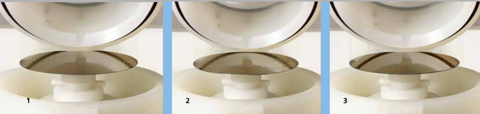
1–3 Coating of a processed wafer with a pre-applicable adhesive via spincoating.
