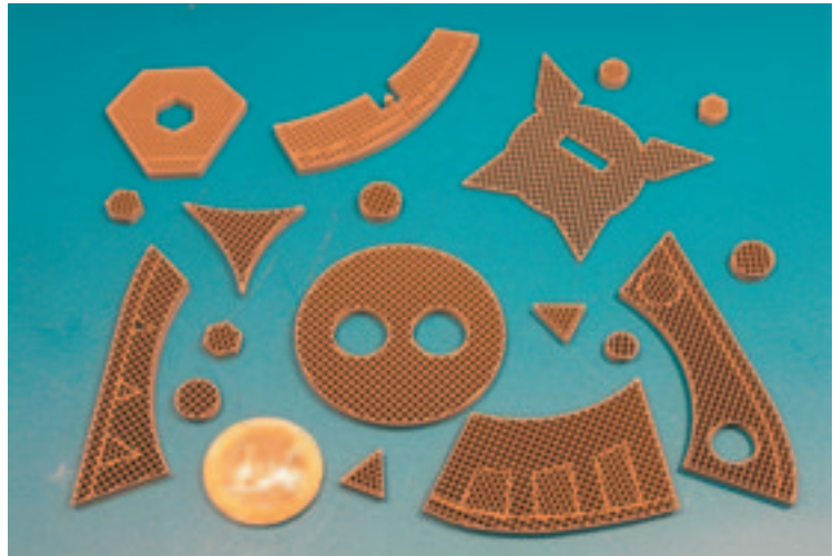
Fig. 5: Cellular direct typing structures made of high-alloy steel.
