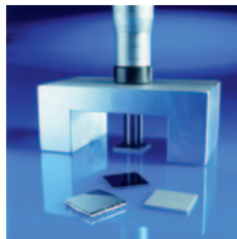
Fig. 3: Device for manufacturing bonded samples with a precisely defined adhesive film thickness.
