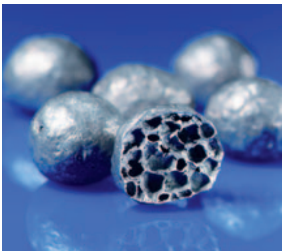
Fig. 1: Cross-section of an APM aluminium foam element.
