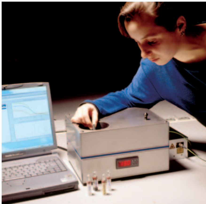
Fig. 4: Light scattering unit developed for measuring the particle size distribution.
