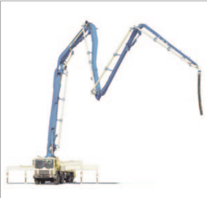
Fig. 1: Concrete pump with extended distribution mast.
