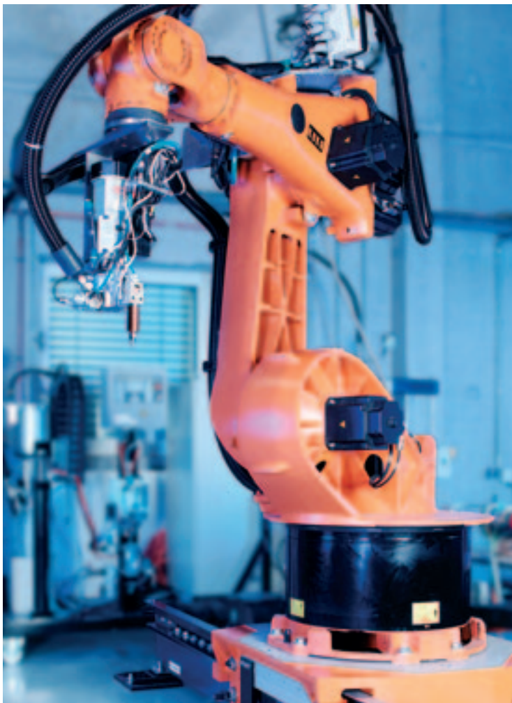
Industrial robot with 1-C piston dosing system.
