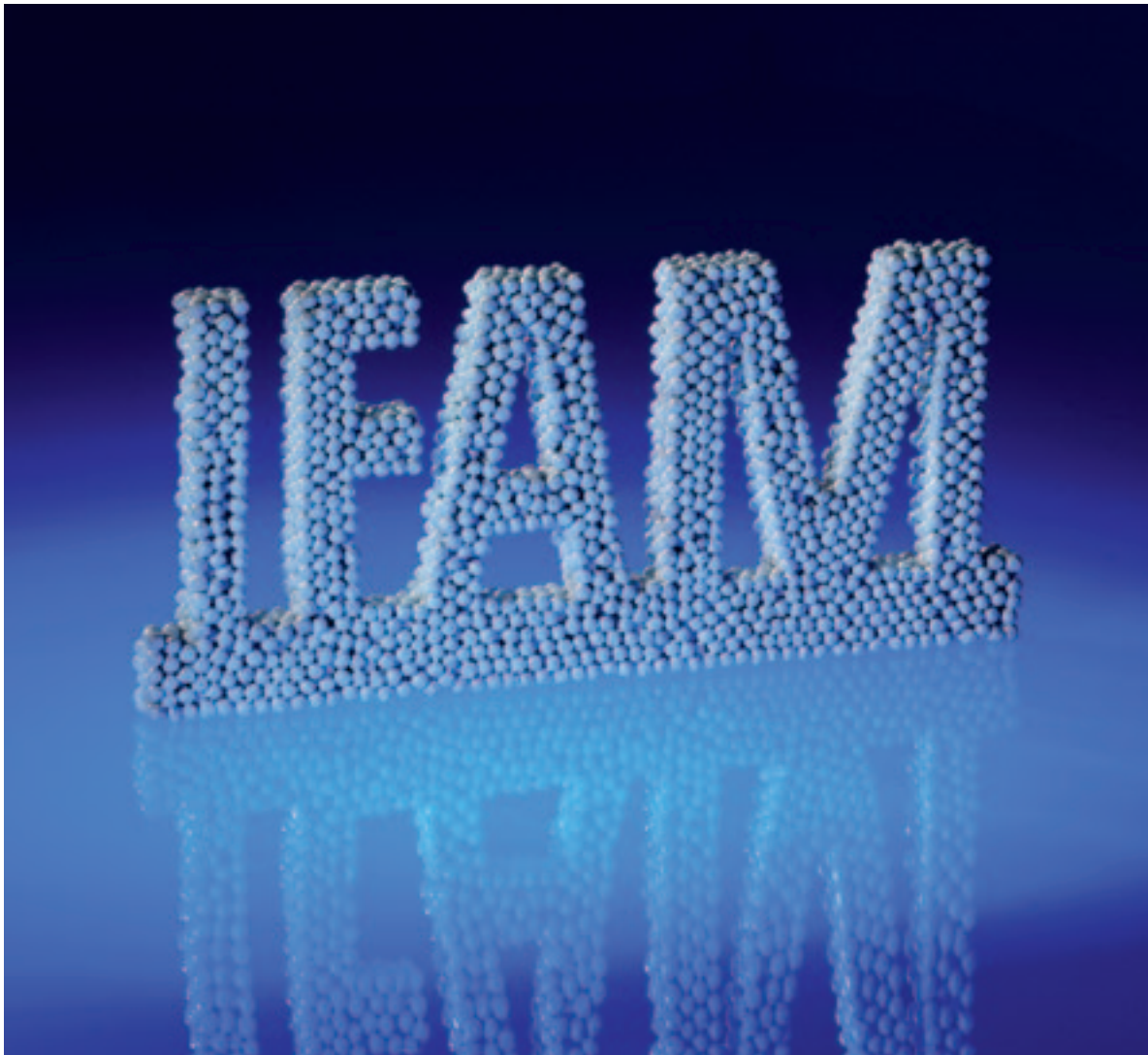
Fig. 4: Design freedom with APM aluminium foam elements.
