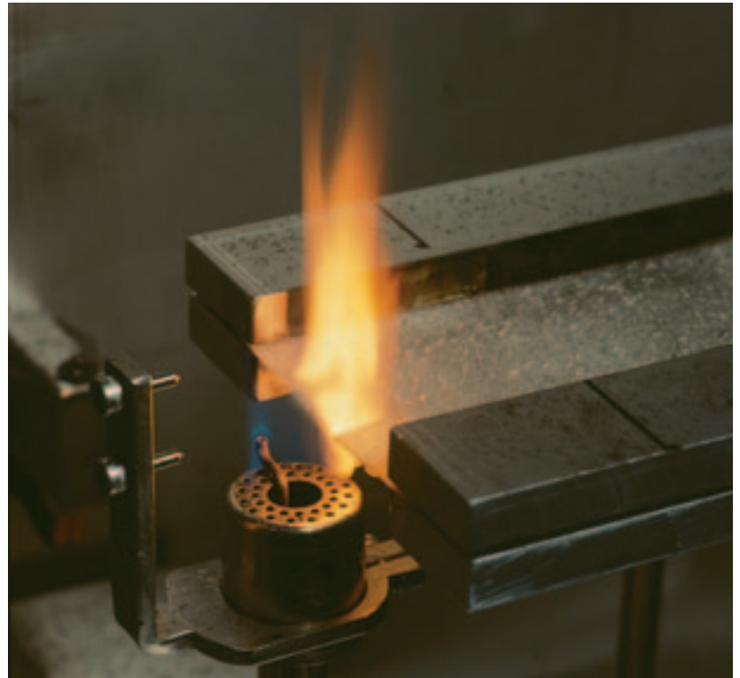
Fig. 2: Flammability test on nanocomposites.
