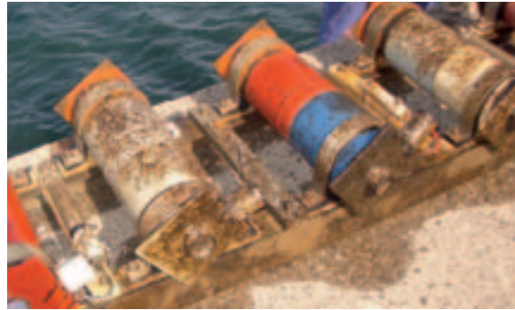
Fig. 4: Practical evaluation of new corrosion protection systems for offshore steel structures. The left figure shows test samples with different coating systems and structural elements prior to exposure to the North Sea at Helgoland. The right figure shows the same samples after 30 months exposure. Except for the left test sample, all samples show clear evidence of corrosion.
