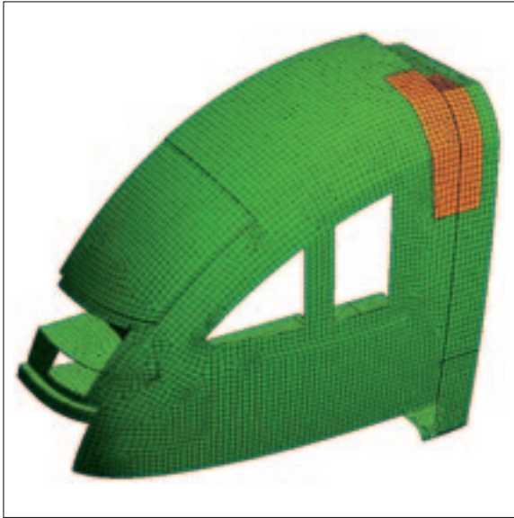
Fig. 2: Model of the front module bonded onto the railcar.
