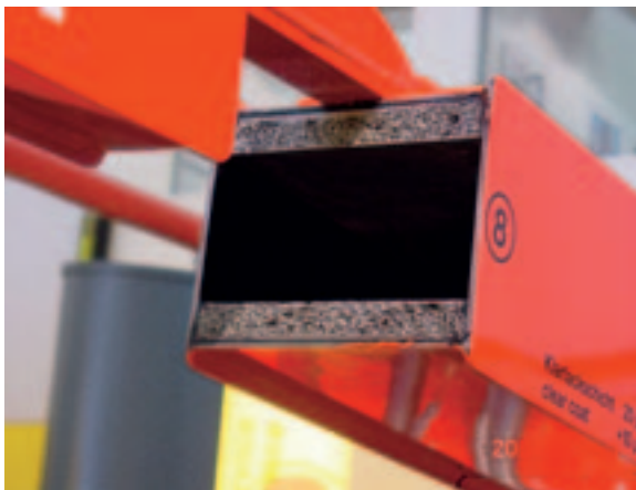
Fig. 2: Demonstration object "concrete pump distribution mast" at the BAUMA 2004 fair (above: overview, below: close-up).
