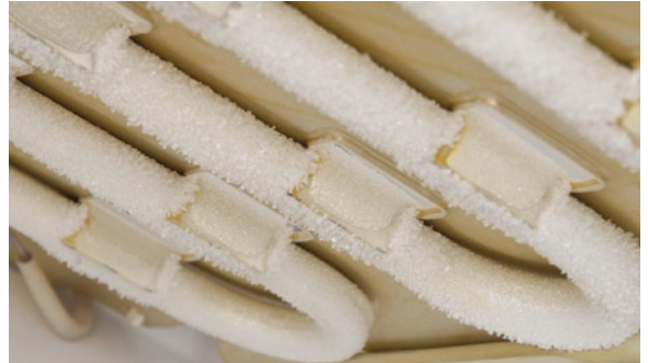
Model of a lacquer surface with antifreeze peptides.
