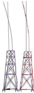
Fig. 4: Second eigenmode of the support structure in ANSYS® (left) and ADCoS (right).
