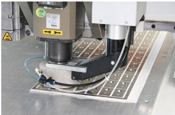
Fig. 3: Hollow sphere structure for sound encapsulation of a high-speed milling cutter.
