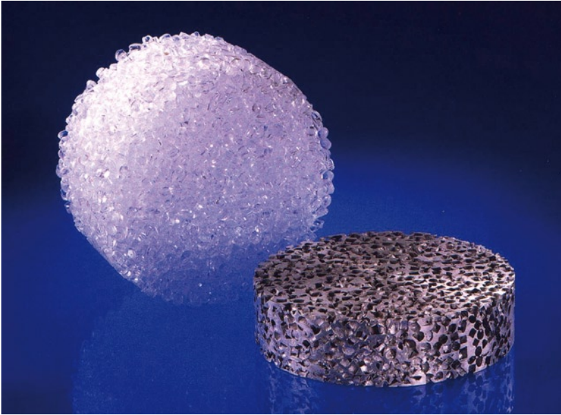
Fig. 1: Placeholder structure of polystyrene granulates and the resulting aluminium sponge.
