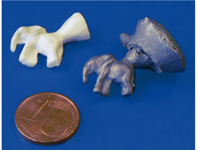
Fig. 4: Demonstrator of an EPS model and a casting.
