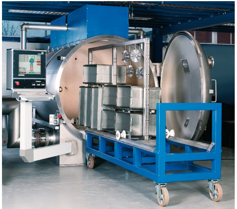
Using this 5 m 3 low pressure plasma plant, components can be coated with PermaCLEAN PLAS® .
