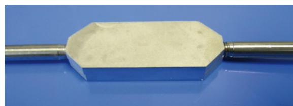
Fig. 6: Co-sintered split-and-recombine mixer with screwed on connections.
