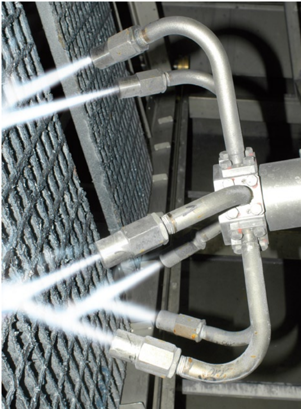
CLAUSwhd paint removal plant with rotating high pressure water nozzles for cleaning gratings (Photo source: Hugo Claus GmbH & Co. KG, Photographer: Britt Moulin).
