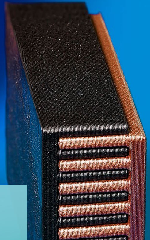
3D printing with thermally highly conductive polymer composite.
