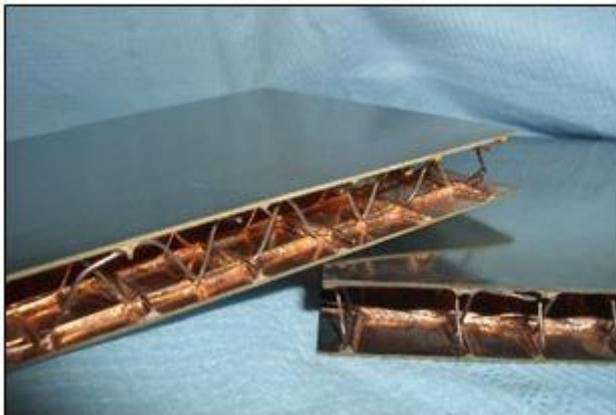
Figure 5: metallic sandwich structure with 3D wire textile core
