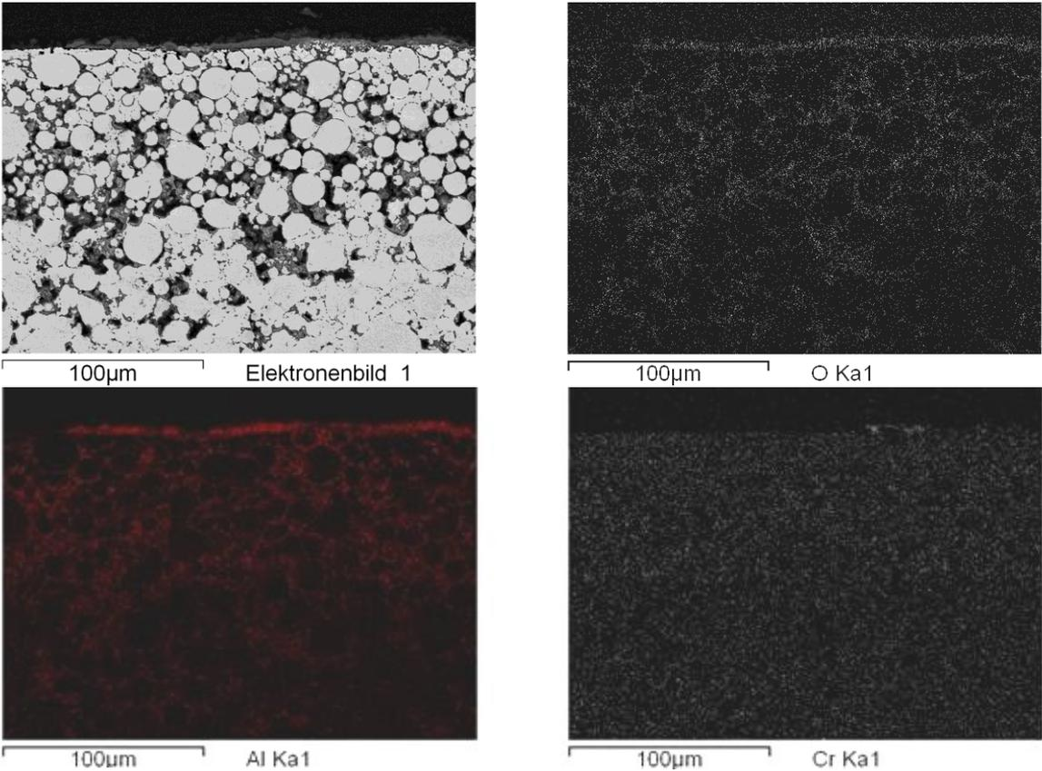
Figure 5: element distribution in alloy IN 713C after isothermal oxidation (900°C, 100h, air)
