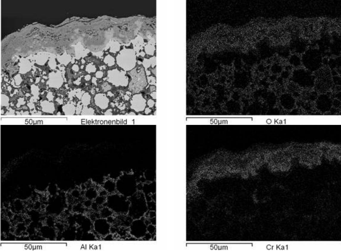
Figure 7: element distribution in alloy IN 713C after isothermal oxidation (1100°C, 100h, air)
