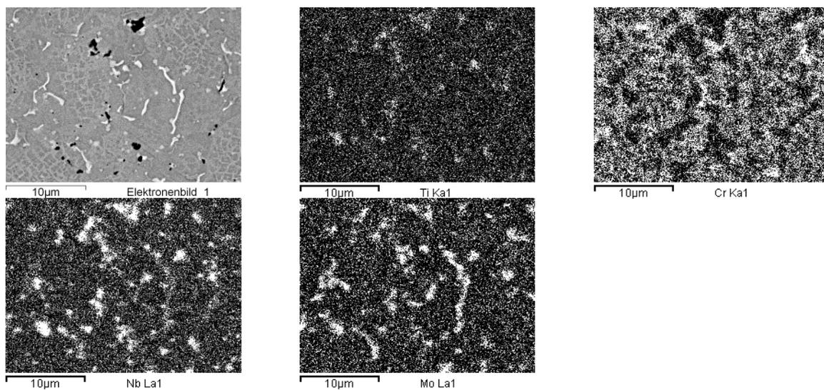
**Figure 3:** element distribution (Ti, Cr, Nb, Mo) in MIM sample of alloy IN713C (condition as sintered)
