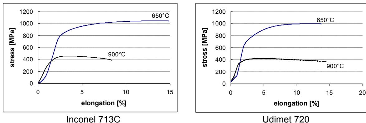
**Figure 2:** typical stress-strain curves at elevated temperatures for alloys of this study
