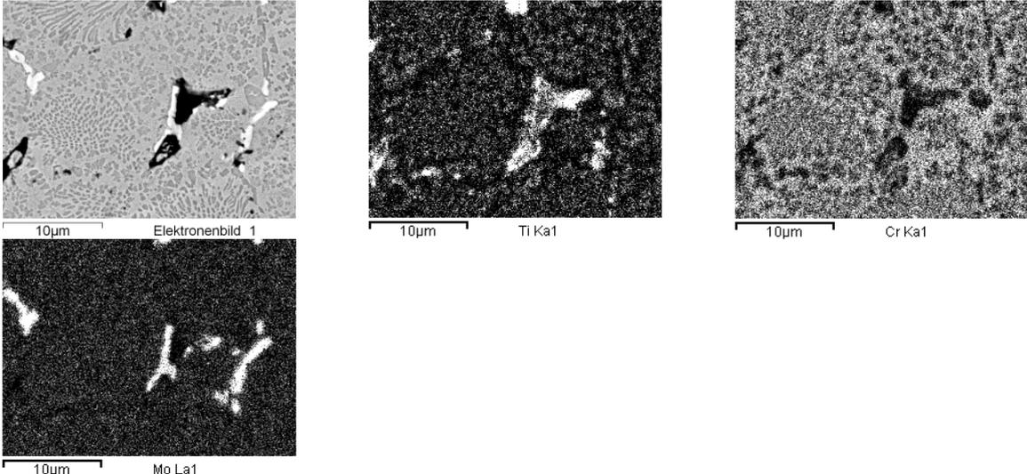
Figure 4: element distribution (Ti, Cr, Mo) in MIM sample of alloy U720 (condition as sintered)
