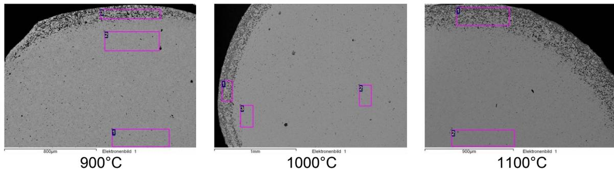
**Figure 8:** SEM images of alloy IN 713C after oxidation for 100h at different temperatures
