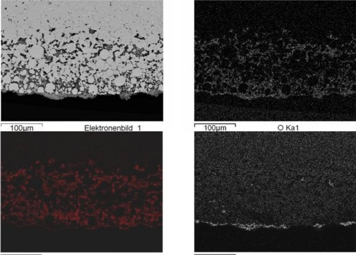
Figure 6: element distribution in alloy IN 713C after isothermal oxidation (1000°C, 100h, air)
