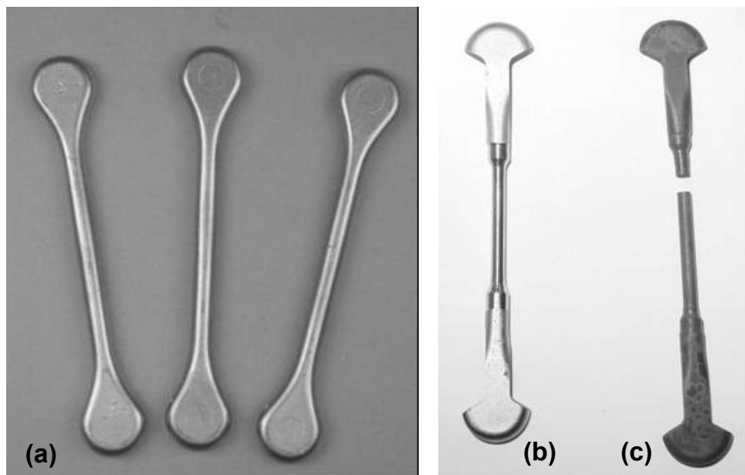
**Figure 1:** (a) MIM tensile bars, (b) MIM tensile bar, machined for HT testing, (c) MIM tensile bar after HT mechanical test (tensile test)
