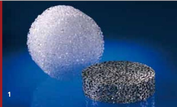
1 *Polymer preform and open porous aluminum foam.*
