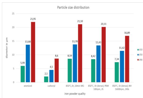
**Figure 2.** Particle size of the reduced and milled powders compared to commercial carbonyl and atomized spherical iron powders
