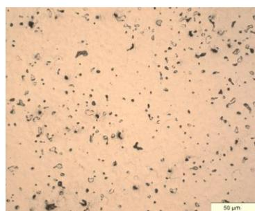
e) reduced and Hybridizer milled for 240s, 16000 rpm
