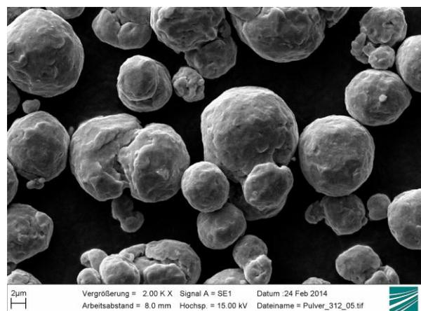
**Figure 3.** SEM image of the powder reduced at 500 °C, 1 h + 850 °C, 1 h H<sub>2</sub>, milled 4 min, 16000 rpm in a Nara Hybridizer (NH),
