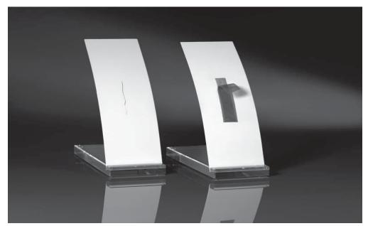
Application of pickling tape prior to the repair of damaged paint. The paint has been removed by mechanical abrasion and the pickling tape is used for pre-treatment of the metal surface. After removal of the tape and simple cleaning with a damp cloth, the surface is ready to receive a fresh coat of paint. (© Fraunhofer IFAM) | Picture in color and printing quality: www.fraunhofer.de/press
