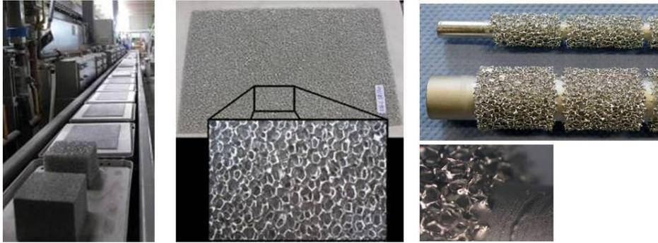
Figure 5: Industrial walking beam furnace with foam tiles and examples of research program (middle: tiles for deflector plates, right: heat exchanger tube with excellent bonding)
