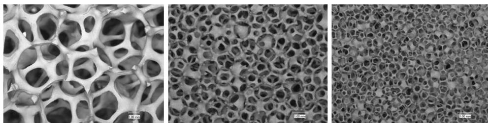
Figure 3: Coated foams; Left: foam with 4.5 mm ecd (ppi 10); middle: 1.0 mm ecd (ppi 45), right: 0.6 mm ecd (ppi 60)
