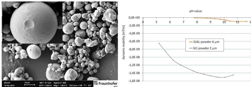
Figure 1: Left: powder morphology of 316L-powder; Right: dynamic mobility of 316L-powder compared to silicon carbide powder
