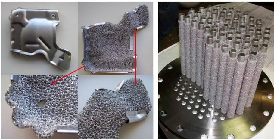
Figure 6: Left: deformed reflector plate (source: Elring Klinger), Right: prototype of a foam heat exchanger (source: Deller GmbH)
