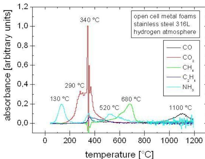
Figure 4: IR Absorption due to the mainly appearing species as a function of furnace temperature
