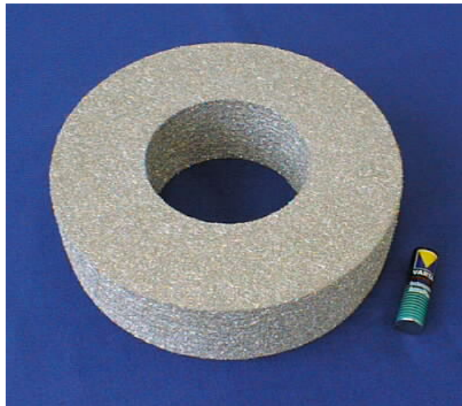
Fig. 3: Heat regenerator prototype for a Stirling machine made from sintered stainless steel fibers (porosity: 85 %)
