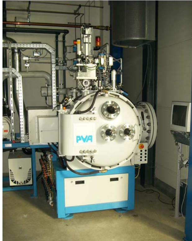
FIGURE 4. New IFAM melt extraction plant allowing for over-pressure of 10 bar
