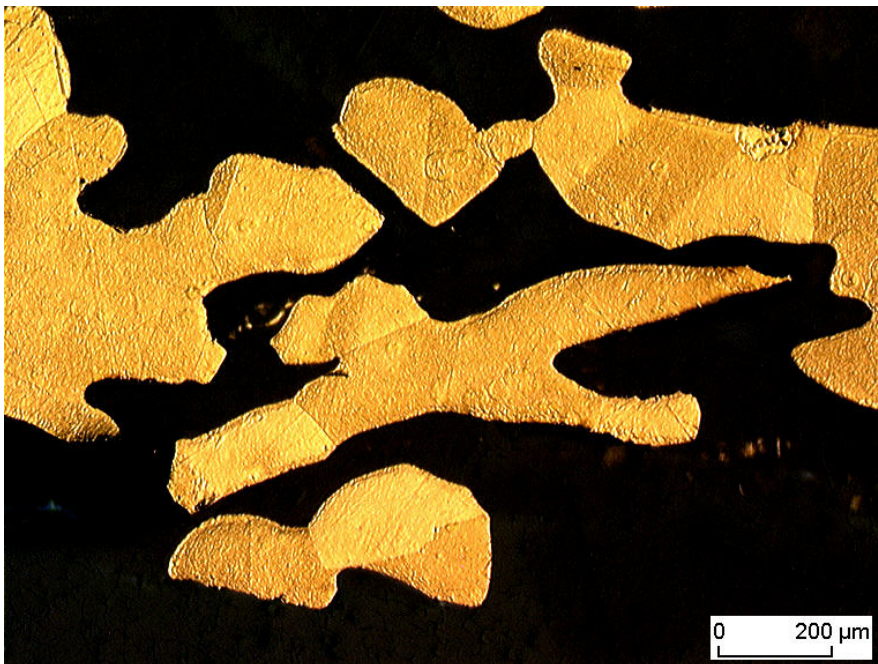
FIGURE 8. Etched cross section of sintered fiber mat made from melt extracted 18 ct. gold fibers (IFAM)
