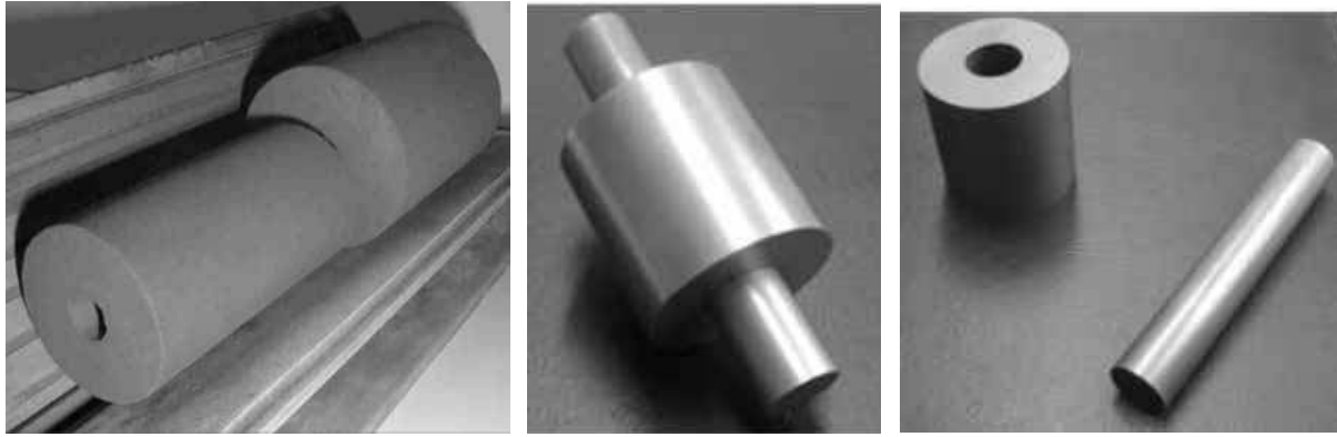
Figure 2: Dies for hot pressing (test pieces): Left cylindric samples after CIP. Middle and right: die and piston after finishing (EMD and surface grinding)
