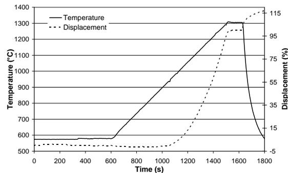
Fig. 3: Displacement and temperature profile for the Spark Plasma Sintering of a  $3\text{Ti/Si/2C}$  powder mixture milled for 1 h.
