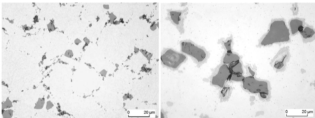
Fig. 8: Optical micrograph (bright field) of spark plasma sintered (left) and hot pressed (right; the sample contains SiC with a different grain size.) Ti6Al4V/15 SiC powder mixtures. Bright phase: Ti6Al4V, dark gray phase: SiC, light gray phase: Ti-Si intermetallics.
