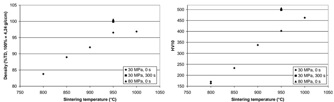
Fig. 7: Density (left) and Vickers hardness HV10 (right) of Ti6Al4V/15 SiC samples densified by SPS/FAST.
