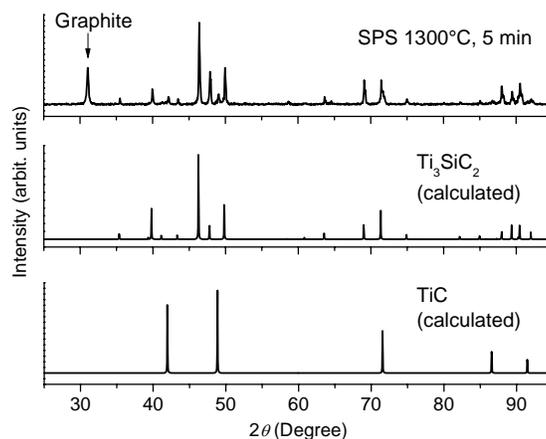
Fig. 6: XRPD patterns of the samples obtained by spark plasma sintering 3Ti/Si/2C mixtures (left). The graphite originates from residual traces of graphite foil used to protect the pressing tool.
