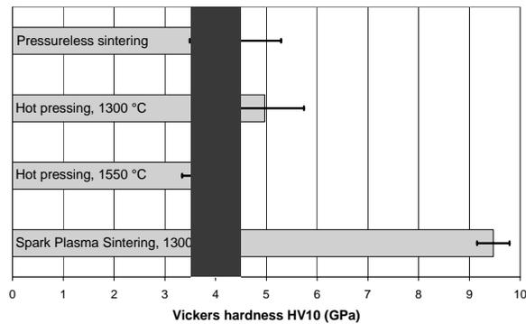
Fig. 5: The Vickers hardness of  $Ti_3SiC_2$  samples sintered by different methods compared with the literature value (gray area between 3.4 and 4.5 GPa) [6].
