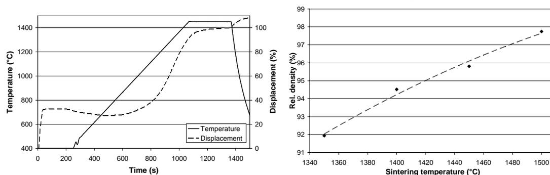
Fig. 1: Temperature and displacement profile for high energy milled  $MoSi_2$  powder mixtures during spark plasma sintering (left). Bulk density of SPS samples as a function of sintering temperature (right).
