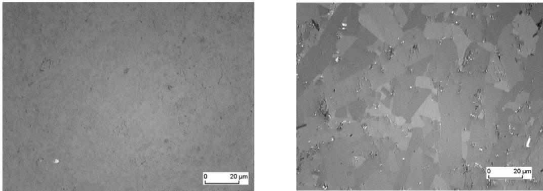
Fig. 4: Optical micrographs (polarized light) of sintered 3Ti/Si/2C powder mixtures (left: spark plasma sintered 1300°C/5 min; right: HP 1550°C/60 min).
