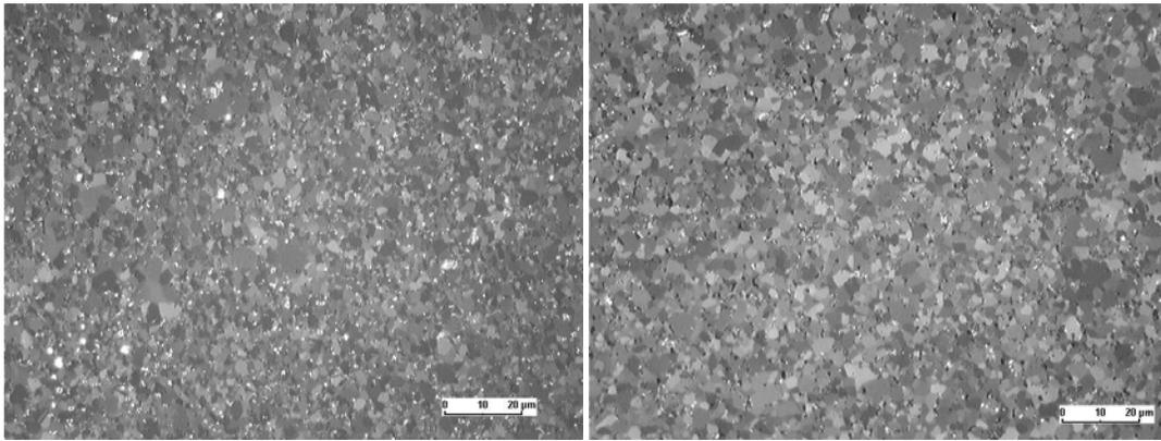
Fig. 2: Optical micrographs of  $\text{MoSi}_2$  samples sintered at  $1400^\circ\text{C}$  (right: SPS, left: Hot pressing) (polarized light).
