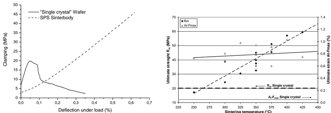
Figure 4: Representative results of 3-point bending tests for coarse crystalline and sintered samples of p-type  $\text{Bi}_{0.5}\text{Sb}_{1.5}\text{Te}_3$  (left). The dependence of the ultimate strain and the ultimate strength with the sintering temperature is shown on the right.
