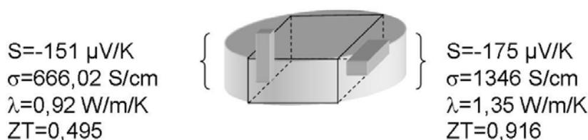
Figure 3: Results of the anisotropic characterization of the physical properties of a spark plasma sintered sample (n-type alloy).
