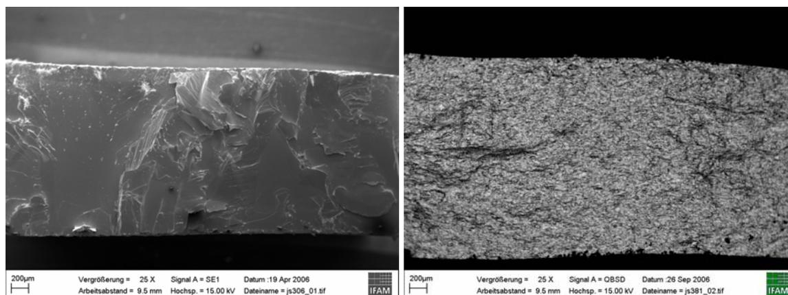
Figure 5: SEM micrographs of the fracture surfaces of 3-point bending bars after mechanical testing. Left: coarse crystalline ingot; Right: Spark plasma sintered powder (400°C/ 1min).
