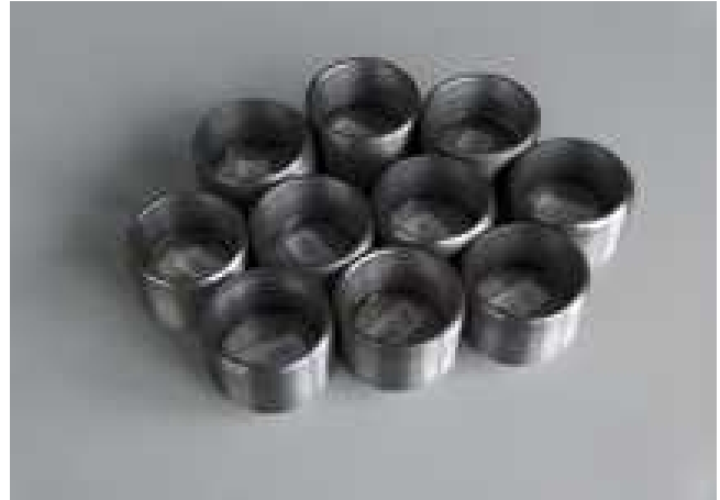
Fig.3 Prototypes of gas inlets for explosion proof gas sensors
