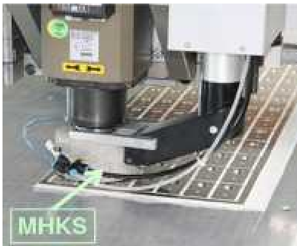
Fig. 1 Metal hollow sphere encasement for high-speed milling tool (courtesy Portatec GmbH)
