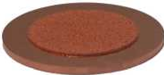
Fig. 1 Metafoam's Copper Foam Boiling Surface
