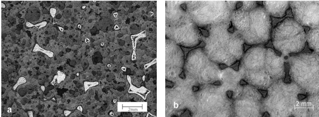
**Figure 3.** hybrid foams with steel host foam, a) interpenetrating DSiC foam (grey, steel: white) b) interpenetration expandable polystyrene foam (white, steel: dark grey)
