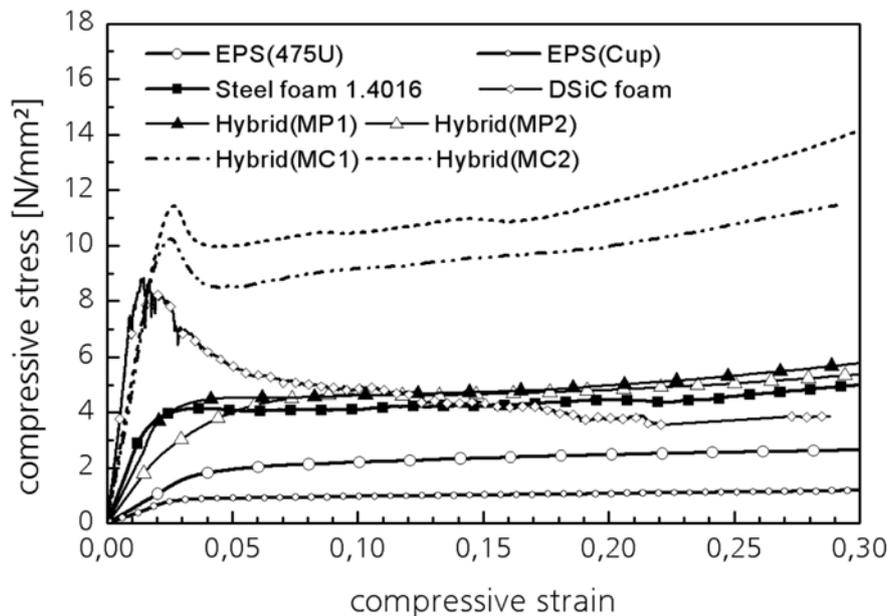
**Figure 4.** typical compressive stress vs. strain curves of the mono material foams and the hybrid foams (Tab. 1); samples: mono-polymer foams: EPS 475U and EPS Cup; mono-ceramic foam; DSiC foam; mono-metal foam: open cell steel foam 1.4016; hybrid foams: metal-polymer: MP1/MP2; metal-ceramic: MC1/MC2
