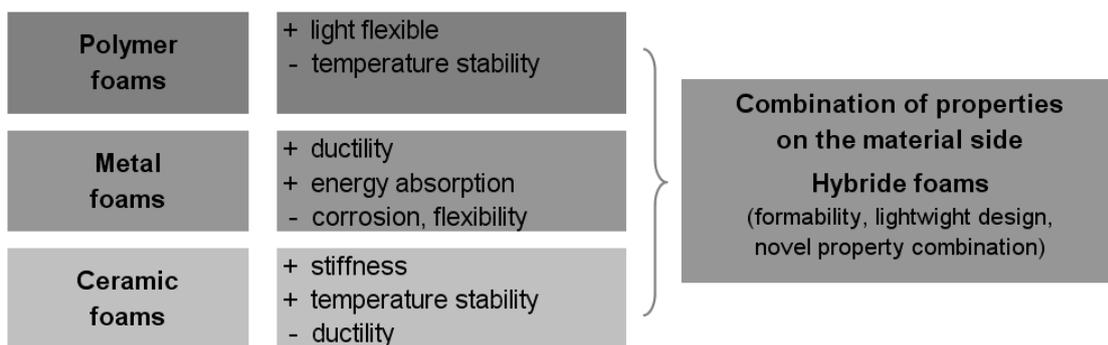
Figure 1. specific properties of the mono material foams
