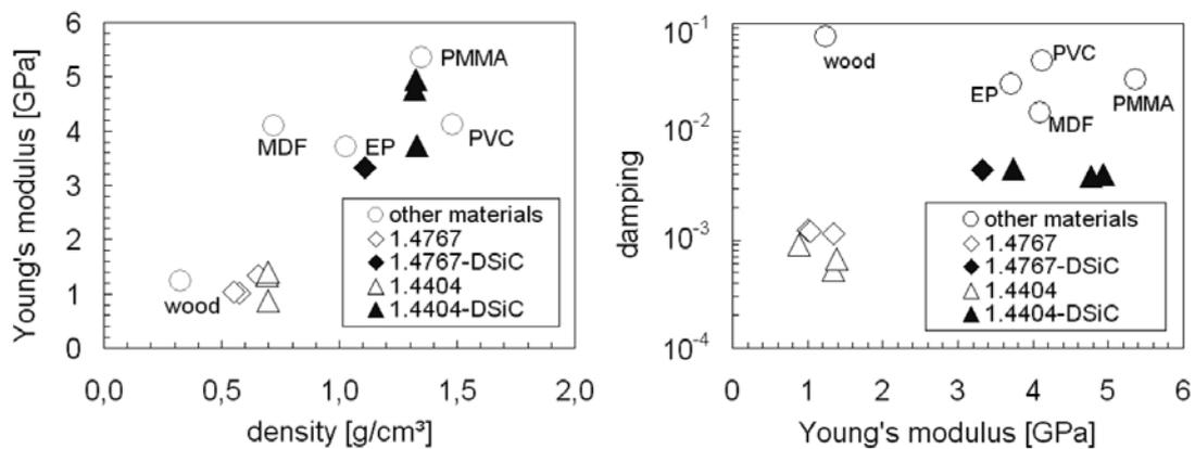
**Figure 5.** results for Young's modulus and damping measured by resonance-frequency-damping-analysis of selected polymers and wooden materials (MDF), open cell steel foam (1.4404 and 1.4767) and same steel foam samples with interpenetrating DSiC
