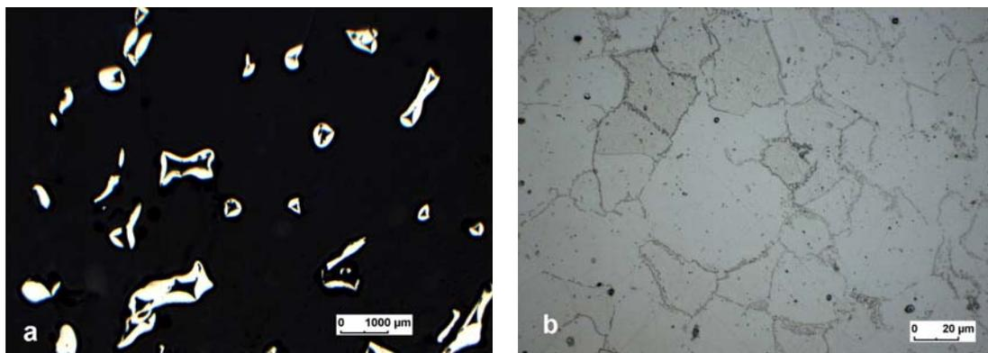
**Figure 2.** micrographs of sintered ( $1280^\circ\text{C}$ ,  $\text{H}_2$ , 1h) open cell 1.4016 steel foam, a) cell struts with typical porosity less then 2%, b) typical microstructure, etched V2A-Beize
