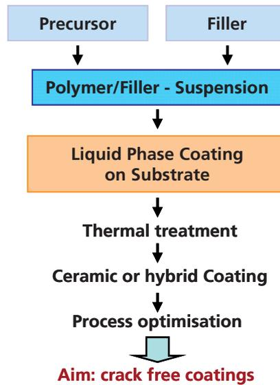
**Figure 1:** General technological steps of Liquid Phase Deposition (LPD).
