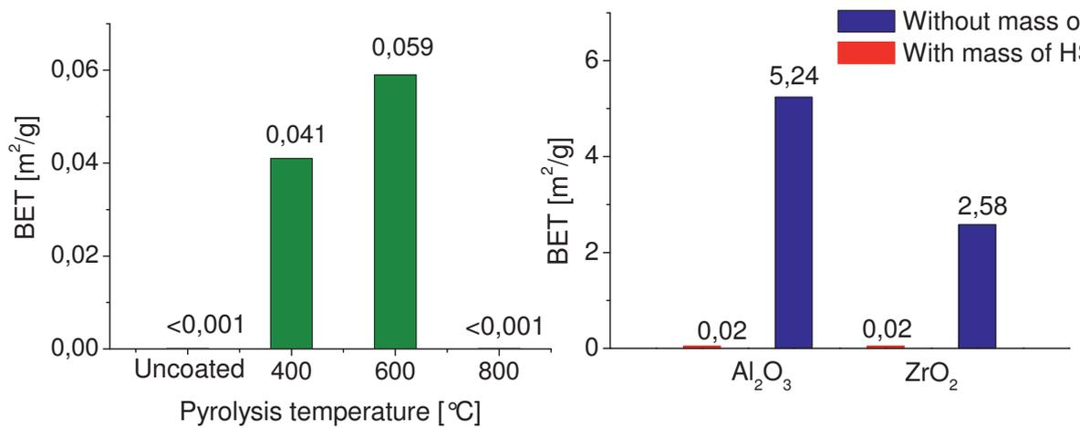
**Figure 4:** a): Temperature effect on BET surface for bioglass coated metallic hollow spheres (316L); b): Comparison of the calculation of the BET surface of porous Al<sub>2</sub>O<sub>3</sub> and ZrO<sub>2</sub> coatings with and without consideration of the mass of the substrate (HS) after annealing at 800 °C.
