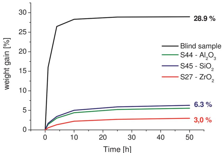
**Figure 6:** Results of Oxidation tests on open celled metallic foam based on carbonyl iron coated with a filled ceramic SiCN coating. (50 h,  $800^\circ\text{C}$ , air).
