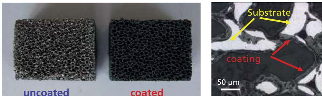
**Figure 5:** Open celled metallic foam based on carbonyl iron coated with a filled ceramic SiCN coating (left); cross section (right).
