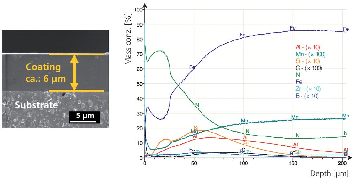
**Figure 2:** Micro structure of a polymer derived ceramic coating (left) and results of GD-OES investigations (right).
