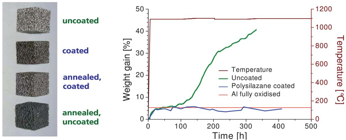
**Figure 7:** Sintered metallic hollow sphere structure based on stainless steel (FeCrAl, 1.4767) coated with a pure ceramic SiCN coating (left); Results of the oxidation test (400 h, 1100 °C, air), (right).
