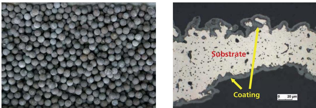
**Figure 3:** Metallic hollow spheres (stainless steel 316L) coated with a bioglass (left) ; cross section (right).
