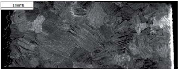
Figure 8: microstructure at the core of the turbocharger after heat treatment
