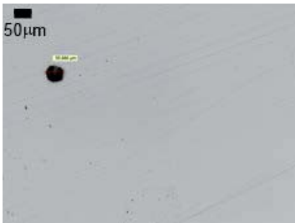
Figure 2: porosity alloy 48-2-2 (spherical pore)
