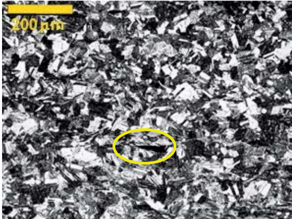
Figure 3: porosity alloy 48-2-2 (elongated pore)
