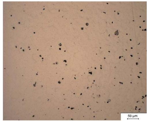
d) reduced 500 °C (932 °F), 1h + 850 °C (1562 °F), 1h + milled 120 min, 100 rpm, ball mill
