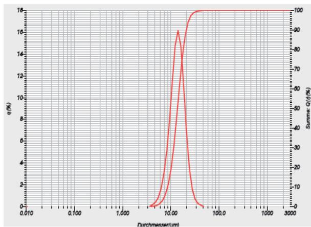
**Figure 5.** Powder reduced at 500 °C (932 °F), 1 h + 850 °C (1562 °F), 1 h under hydrogen and milled for 20 min, 75 rpm in a mortar grinder (MG), a) SEM image, b) particle size distribution
