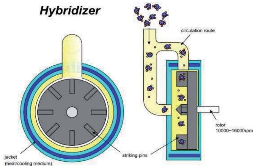
**Figure 2.** Scheme of the grinding process in the Nara Hybridizer
