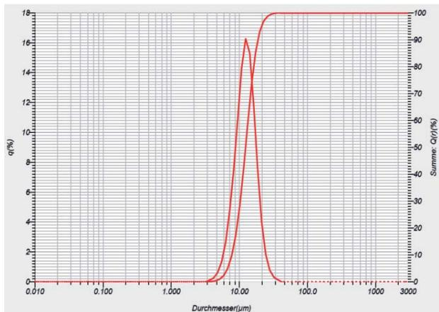
**Figure 6.** Powder reduced at 500 °C (932 °F), 1 h + 850 °C (1562 °F), 1 h under hydrogen and milled for 120 min, 100 rpm in a ball mill, a) SEM image, b) particle size distribution
