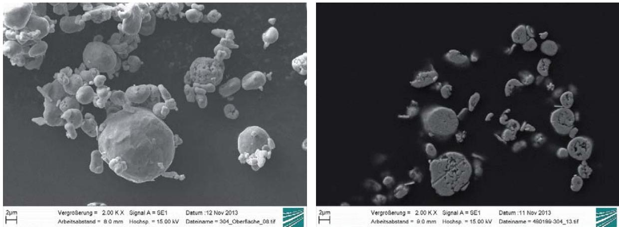
**Figure 9.** Powder reduced at 500 °C (932 °F), 1 h + 700 °C (1292 °F), 24 h under hydrogen and milled for 4 min, 16000 rpm in a Nara Hybridizer (NH),
