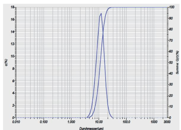
**Figure 8.** Powder reduced at 500 °C(932 °F), 1 h + 850 °C (1562 °F), 1 h under hydrogen and milled for 4 min, 16000 rpm in a Nara Hybridizer (NH), a) SEM image, b) particle size distribution
