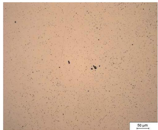
f) reduced 500 °C (932 °F), 1h + 700 °C (1292 °F), 24h + milled 4 min, 16000 rpm
