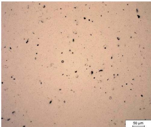
c) reduced 500 °C (932 °F), 1h + 850 °C (1562 °F), 1h + milled 20 min, 75 rpm, mortar grinder
