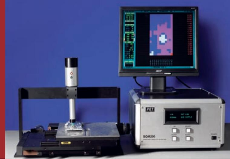
Identification of residual contamination on an aluminum pressure-cast component using Optically Stimulated Electron Emission (OSEE).
