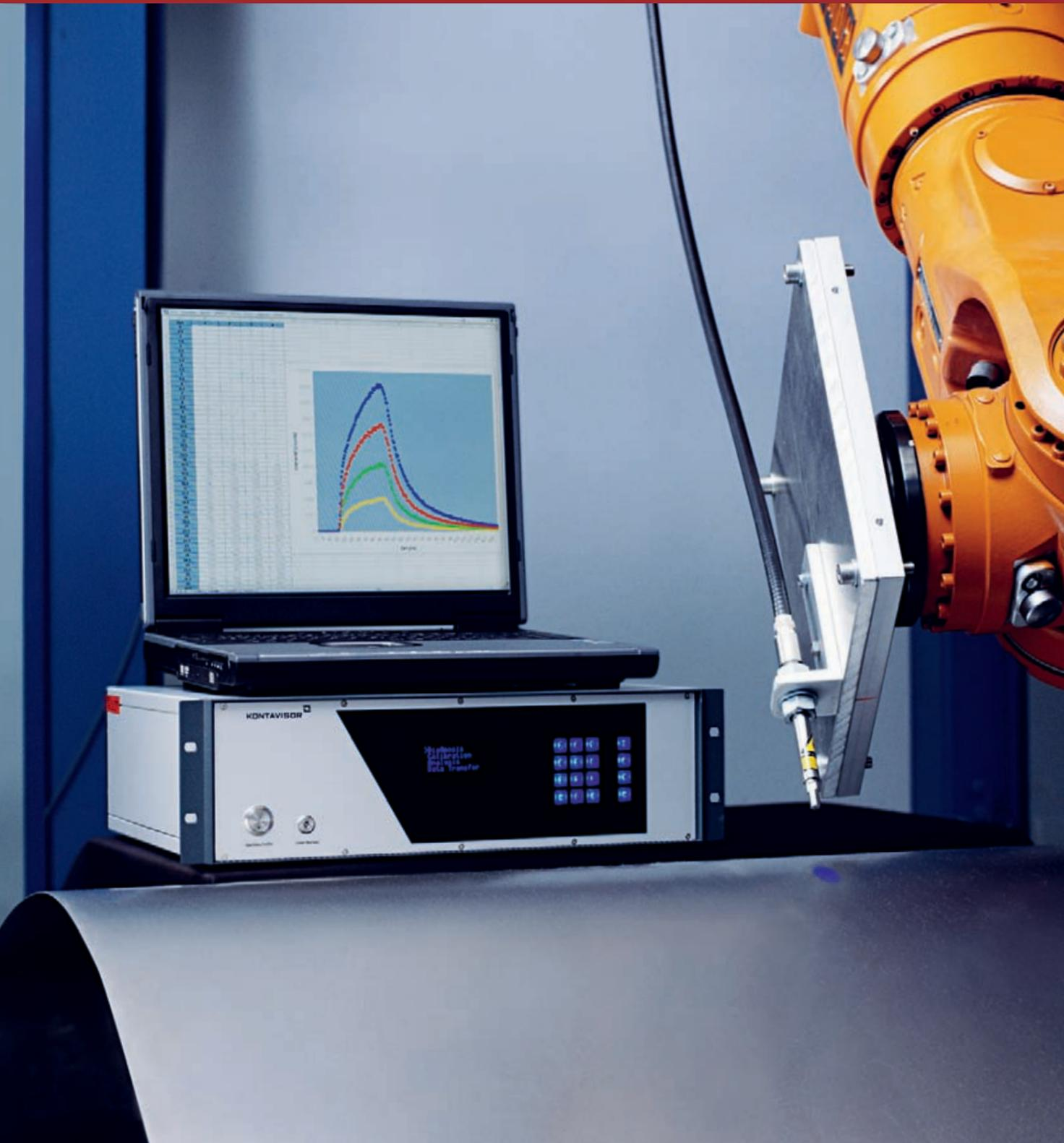
Laser Induced Breakdown Spectroscopy (LIBS) for determining the elemental composition of a sample surface.
