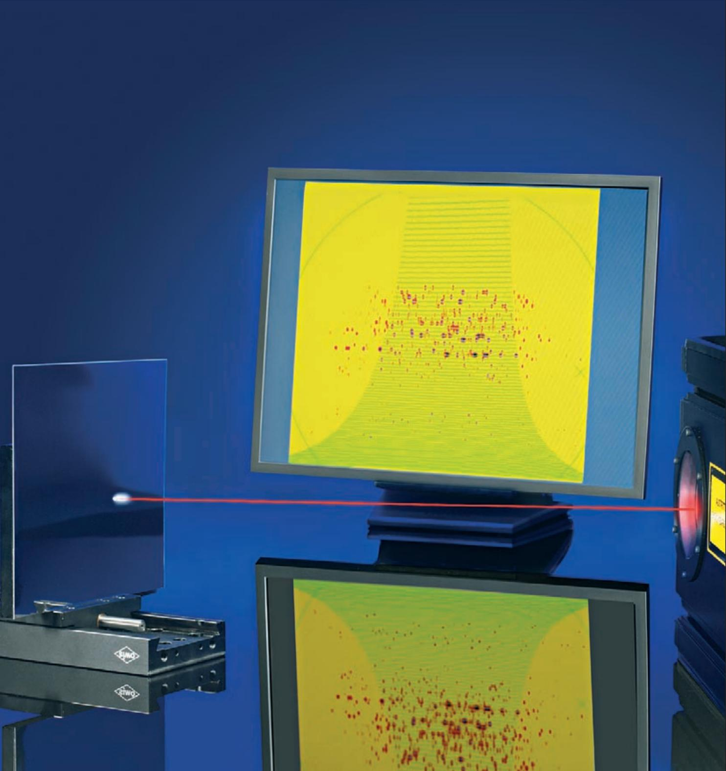
Investigation of the wetting properties of surfaces using the aerosol wetting test: Laboratory test set-up.
