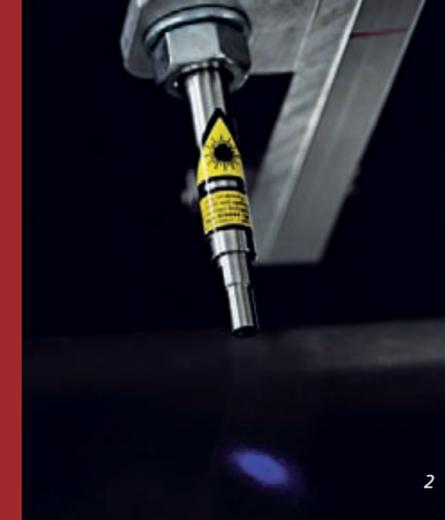
1 Characterization of thin surface films using ellipsometry.
