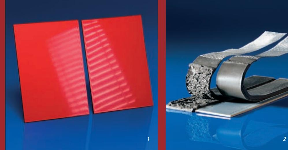
1 Left: defective coating – orange peel effect on a painted surface; right: defect-free coating.
