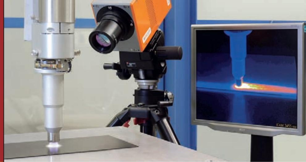
Thermography for monitoring automated pretreatment using atmospheric pressure plasma.
