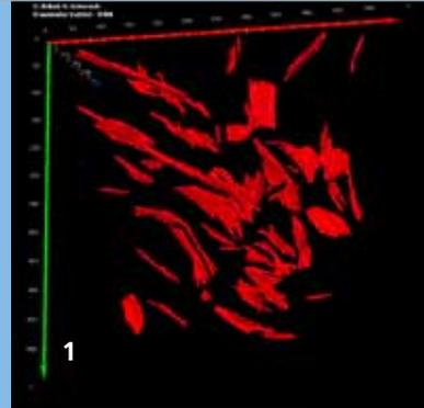
1 3D TEM image of a layered silicate perfectly distributed in an epoxy resin.
