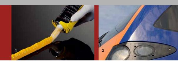
1 Manual application of a moisture-curing polyurethane adhesive from a cartridge.
