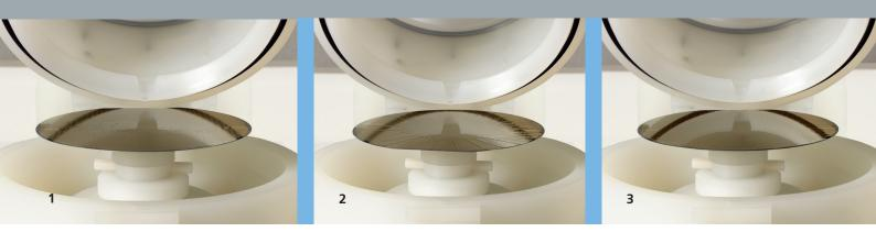
1-3 Coating of a processed wafer with a pre-applicable adhesive via spincoating.
