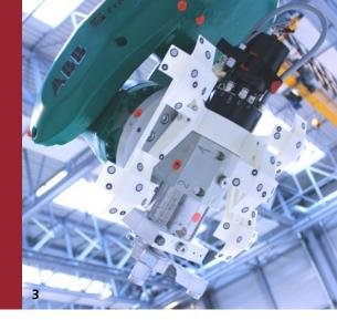
parameters (e. g. temperature) – this enables a **static positioning accuracy** of **better than 0.1 mm** to be achieved in the entire workspace. This technology is therefore particularly suitable for high-precision drilling applications of large components.
