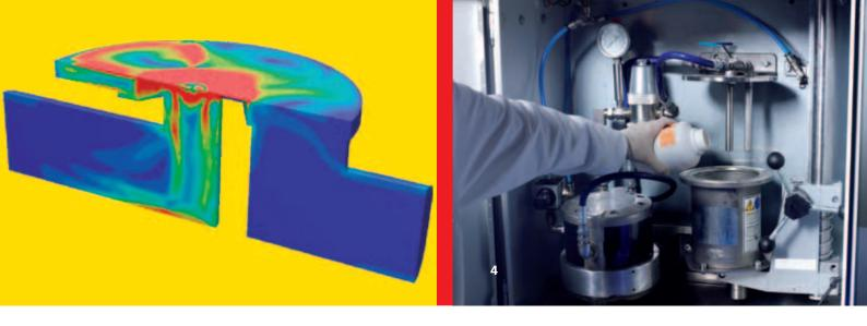
The paint/lacquer can be passed through this loop system either continuously or intermittently. The test loop can be heated up to 40 °Celsius.
