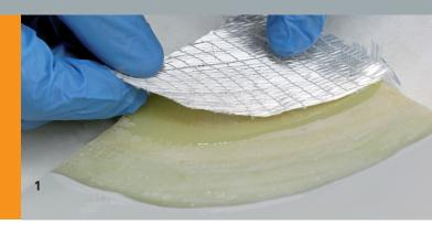
Reconstruction of the layer structure for the repair of a glass fiber composite – skills learned in the FRP-Remanufacturer training course at the Fraunhofer IFAM.
