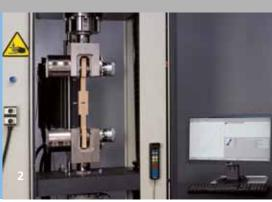
Adhesively bonding: Small specimens are used for determining the wood strength, medium-sized lap shear specimens are used to select adhesives, and large specimens are used to verify the results on components.
