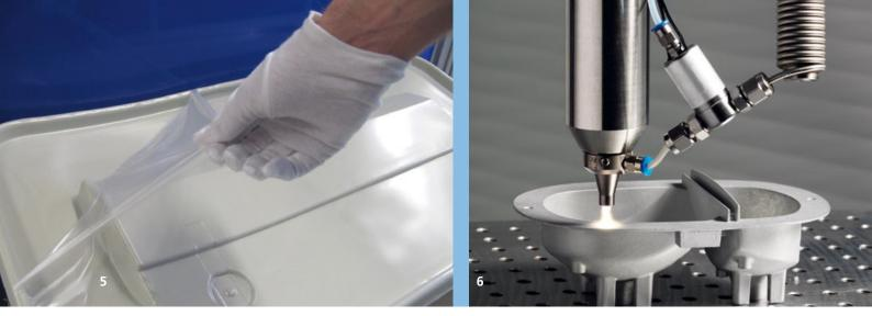
involves three steps – namely the molding of the component, the removal of release agent residues, and the application of a scratch protection coating – the process developed at Fraunhofer IFAM allows a component to be manufactured in a single step. Here, the film remains on the manufactured component for protection right to the end of the process or even up to delivery to the end customer, potentially saving further processing costs and work steps.
