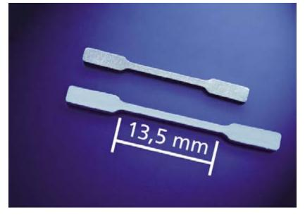
Fig. 6: Micro tensile test specimen: Green component and sintered component.
