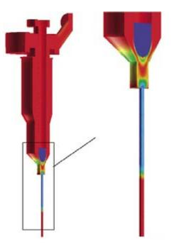
Fig. 3: Pressure of the adhesive in the valve nozzle with an open valve.
