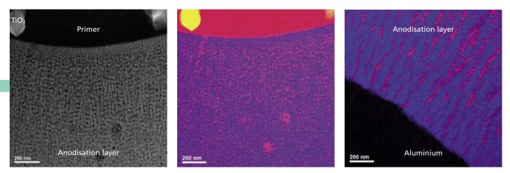
Fig. 3: TEM image of a primer-treated aluminium anodisation layer. The carbon distribution in the corresponding elemental map (carbon – red, oxygen – blue, titanium oxide – yellow) shows that the primer penetrated into the pores down to the aluminium substrate.
