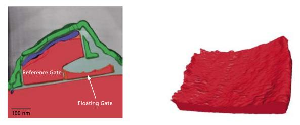
Fig. 6: Surface rendering of the 3-D structure of a flash memory cell (Si – red,  $SiN_x$  – green,  $TiSi_x$  – blue); the right side shows the surface roughness of the floating gate.
