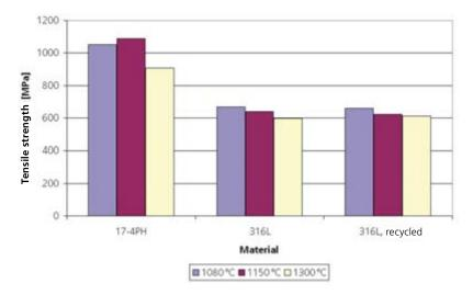
Fig. 7: Tensile strength of micro tensile test specimens (316L and 17-4PH) after sintering at different temperatures.
