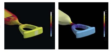
**Fig. 3:** Simulation of temperature distribution and mould filling behaviour for micro metal injection moulding.
