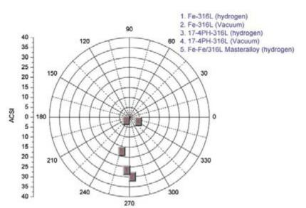
**Fig. 1:** ACSI (apparent co-sintering index) for five different variants for manufacturing a magnetic – non-magnetic combination of materials. Combinations 3, 4 and 5 have ACSI values < 15 and have been successfully manufactured.
