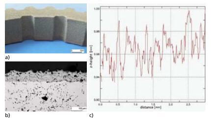
Fig. 2: Sprayed on molybdenum lining on a synchronizer ring, a) plan view, b) crosssection and c) in profile.
