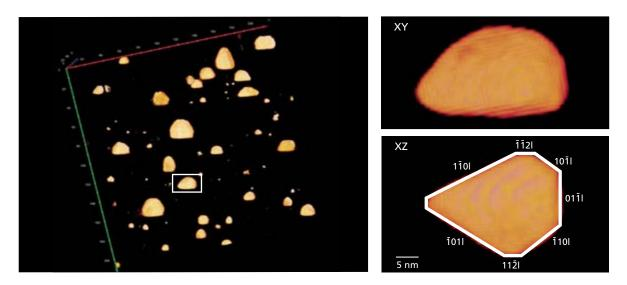
**Fig. 7:** Volume rendering of  $ErSi_2$  nanoparticles having a diameter of 1-20 nm. The close-up on the right side shows a particle from two different directions, revealing the well-defined facets observed for these crystals. Sample courtesy of Prof. U. Kaiser, University of Ulm.
