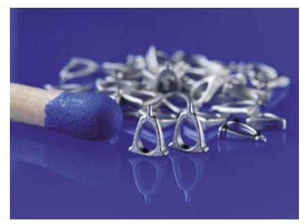
Fig. 8: Series production of stirrup made of 316 (cooperation with Krämer Engineering, Rendsburg).
