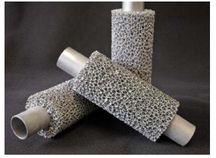
**Fig. 4:** Composite structures made from steel tubes and steel foam (steel grade 316L, cell width 20 ppi) for use as air heat-exchangers. By shrinking the foam onto the tubes, the surface area of the tubes is greatly increased.
