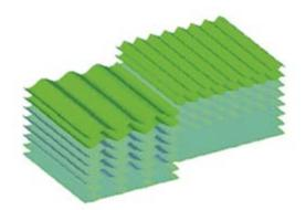
**Fig. 2:** Penetration of surface waves into a film (light green) – substrate (pale green) system. Front – long wavelengths; Back – short wavelengths.
