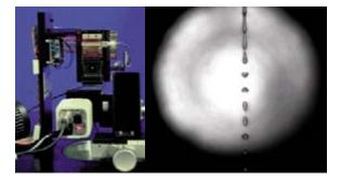
**Fig. 3:** Ink-jet print head test station for visualisation of the formation of drops of functional inks.
