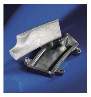
Fig. 2: Foam core for the A-pillar.
