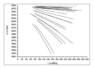
Fig. 6: Dispersion curves of PS films on Si wafers. The virtually horizontal line represents the non-coated substrate. The lowermost line represents a PS film of ca. 1  $\mu$ m thickness.
