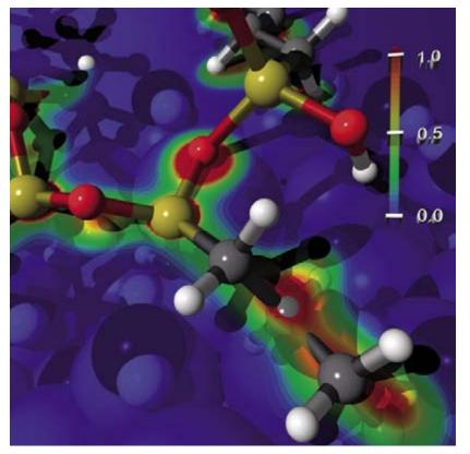
**Fig. 3:** Representation of the calculated electron density distribution in the surface region when components of an adhesive come in contact with an aluminium substrate. The colour-scale indicates the distribution of the electron density in the surface region.
