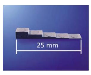
Fig. 4: Moulded sample: micro-steps.
