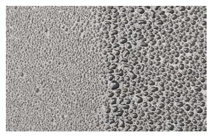
**Fig. 5:** Wetting properties of plastic surfaces. Left: Non-pretreated region of a sample surface; Right: Pretreated region with improved wetting properties.
