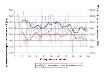
Fig. 5: Relationship between the internal pressure in the mould and component weight for micro injection moulding.
