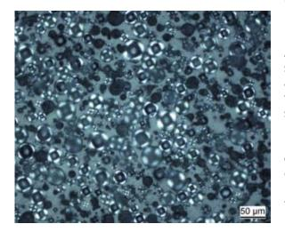
**Fig. 2:** Composite material based on metals and microscopic small glass bubbles produced by casting. The maximal size of the glass bubbles is 60 microns.
