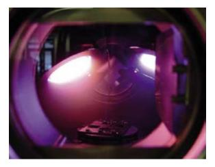
Sputter technology for nanostructured, functional layers.
