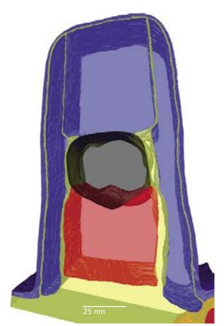
Fig. 1: 3-D representation of the structure of a transistor in a DRAM memory device showing the roughness of the hidden interfaces and enabling 3-D metrology (Si – red, SiO<sub>X</sub>/SiO<sub>X</sub>N<sub>y</sub>– yellow, SiN<sub>y</sub> – blue, WSi<sub>X</sub> – black).
