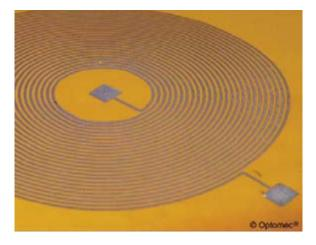
**Fig. 1:** "Functional Printing": Maskless printing by using the Maskless Mesoscale Material Deposition (M<sup>3</sup>D) process. Silver micro-antenna on flexible substrate.
