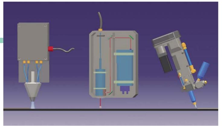
Fig. 3: Schematic representation of the in-line monitoring of surface quality in an automated bonding process. From left to right: Pretreatment of the surfaces via plasma pretreatment, in-line monitoring of the surface quality, adhesive application.
