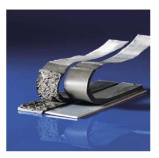
**Fig. 2:** The left-hand sample shows a cohesion fracture in an adhesive film. The right-hand sample shows an adhesion fracture caused by a release coating developed at the Fraunhofer IFAM.
