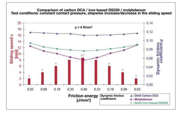
Fig. 4: Results of the stepwise sliding speed test for determining the friction coefficient.
