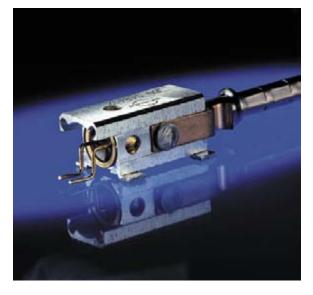
Fig. 1: Micro-bond: VCSEL diode bonded into an SMD housing.
