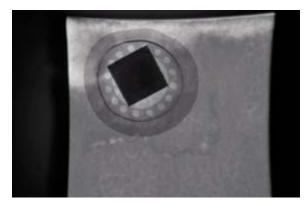
Fig. 3: X-ray image of an integrated RFID: TAG ID 700.
