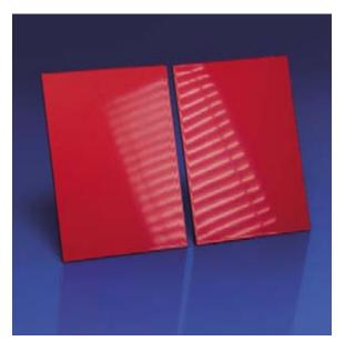
**Fig. 1:** On the left a defective paint surface: Orange peel formation on a painted surface, on the right a faultless paint surface.
