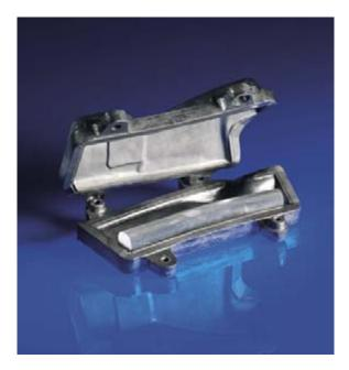
Fig. 1: Semi-finished product in the foam mould.
