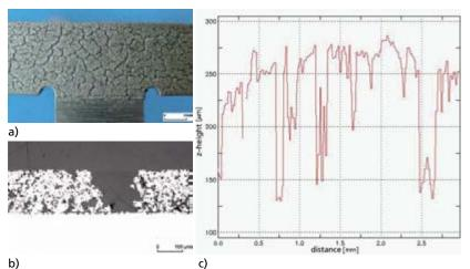
**Fig. 3:** Double cone synchronizer ring with the new iron-based friction lining DS 230, a) plan view, b) cross-section and c) in profile.
