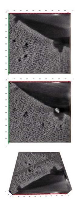
**Fig. 4:** Digital slices through the volume of the anodisation layer show details of the pore structure and clearly show structural defects.
