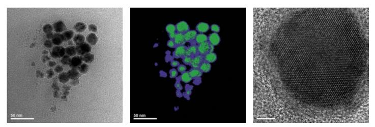
**Fig. 2:** TEM image of a cluster of Co/CoO core-shell nanoparticles. Multivariate analysis of the corresponding Co and O elemental maps shows the Co (green) and CoO (blue) distribution within the particles. Sample courtesy of Prof. A. Wei, Purdue University.
