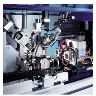
Battenfeld Microsystem 50: Series production plant for micro-components and micro-structured components.
