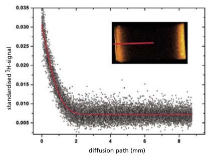
**Fig. 6:** Experimentally determined moisture profile for the penetration of water into a bonded joint. The experimental curve was determined using tracer-studies via ToF-SIMS (Time-of-Flight Secondary Ion Mass Spectrometry).
