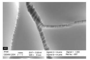
**Fig. 5:** SEM micrograph of a ca. 9 nm thick PS film on an Si wafer generated by spin-coating.
