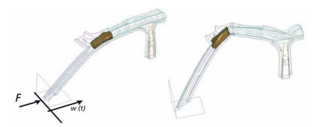
Fig. 3: Position of the aluminium foam core in the A-pillar as determined by virtual optimisation.
