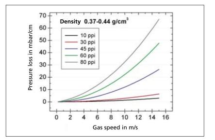
**Fig. 3:** Permeability of open-celled metal foams. The pore width has a large effect on the passage of materials through the pore structure.
