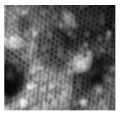
Fig. 1: Electron micrograph (HRSTEM) of zeolite MCM-41. The hexagonal pores in the material can be seen as a honeycomb-like structure. The light areas are larger particles of tin oxide (Sample: M. Wark, University of Hannover).
