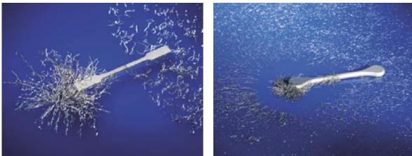
**Fig. 2:** Micro-MIM tensile test sample made from a combination of 316L and 17-4PH. The left part of the sample made of 17-4PH was magnetised and attracts the iron filings. The right part of the sample remains non-magnetic.
