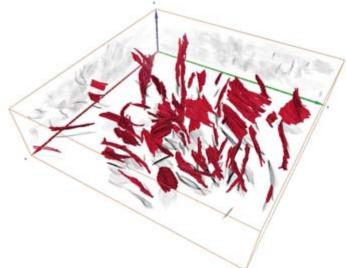
**Fig. 5:** Traditional TEM image of separated organobentonite layers in an epoxy resin. The 3-D reconstruction reveals the shape and distribution of the nanoparticles.
