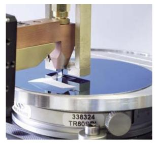
Fig. 4: Measuring head of the LAWave<sup>®</sup> device.
