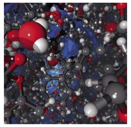
**Fig. 5:** Molecular model for the transport of water in a polymer coating. The polymer is represented using a ball-and-stick representation and balls were chosen to represent the water molecules.
