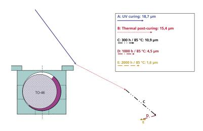
Fig. 3: Misalignment measurement on a non stress-optimised bond.
