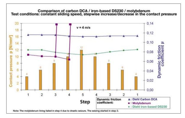
Fig. 5: Results of the stepwise contact pressure test for determining the friction coefficient.
