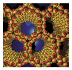
**Fig. 2:** Computer model of the hexagonal pores in zeolite MCM-41.
