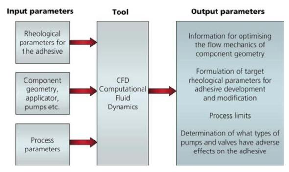
Fig. 1: Input and output parameters for the CFD simulation of adhesive processing.
