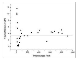
Fig. 7: E-moduli of thin PS films on Si wafers. Full line: bulk E-modulus of polystyrene.
