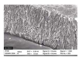
Fig. 9: SEM micrograph of an anodisation layer on aluminium.
