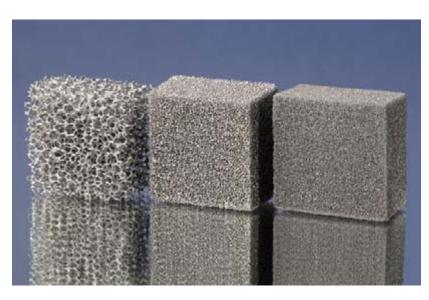
Fig. 2: Open-celled metal foams made from steel grade 316L and having cell widths of 20, 45 and 60 ppi.
