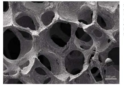
Fig. 1: Scanning electron micrograph of an open-celled structure made from steel grade 316L and having a cell width of 60 ppi.
