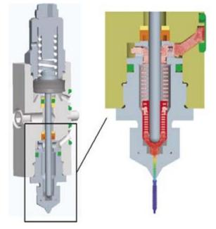
Fig. 2: Cross-section of a dosing nozzle for processing hotmelts.
