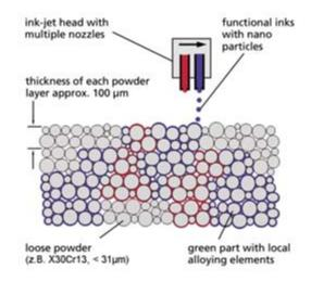
**Fig. 1:** Schematic representation of the manufacture of gradient structures using 3-D-Printing.
