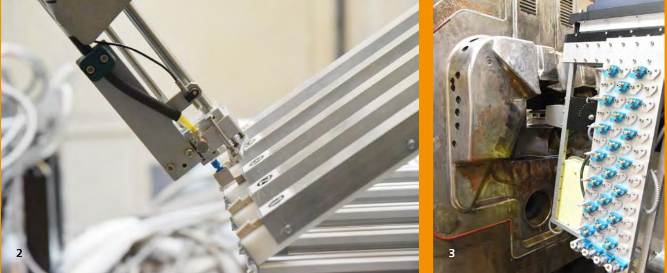
magazine above the die-casting system by a gripper attached to a release-agent-spraying robot and then placed in the mold after the release agent was applied. Immediately after the component was cast and cooled, the transponder was tested for readability and the individual unique code of the transponder was linked to the casting parameters of the cast. All data and parameters could now be traced to the unique component of "batch size 1". Deburring was carried out as the final step.
