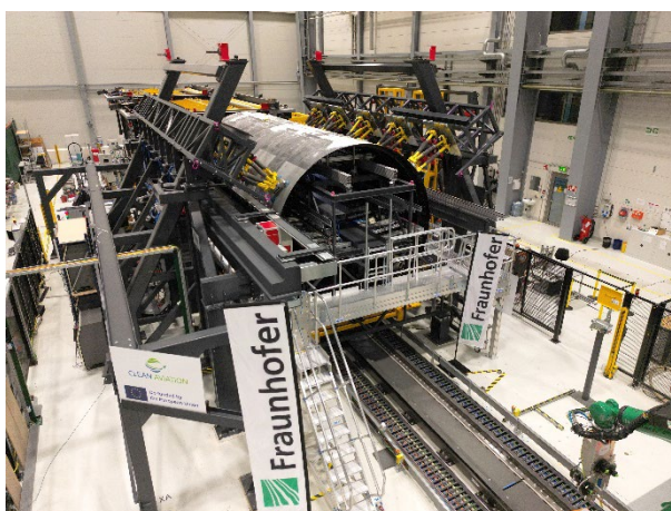
Fig. 1 Assembly research platform with thermoplastic fuselage shells of the MFFD at Fraunhofer IFAM in Stade.
