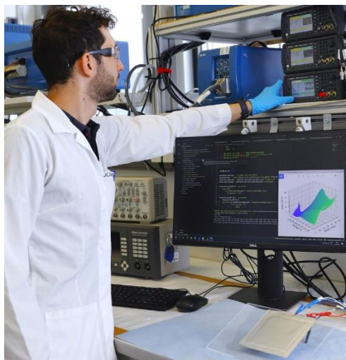
Fig. 1 Lab setup for computer-assisted real-time measurement of impedance in a lithium-ion battery cell to analyze its state.
