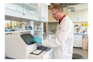
Testing the effectiveness of antiviral surfaces by means of quantitative real-time PCR analysis (qPCR) at Fraunhofer IFAM. © Fraunhofer IFAM
