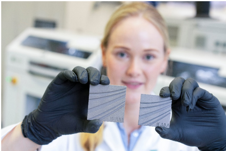
Parts produced by metal binder jetting before (left) and after (right) sintering. © Fraunhofer IFAM
