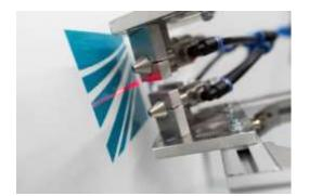
Laser paint stripping in combination with CO<sub>2</sub> snow cleaning for selective decoating and cleaning of ablation products. © Fraunhofer IFAM
