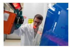
Use of inline hyperspectral cameras for reliable detection of paint buildup in the aerospace industry. © Fraunhofer IFAM
