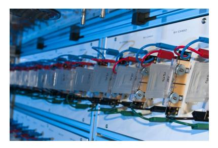
By measuring the so-called dynamic impedance of the battery cells the state of the battery cells during charging can be determined directly. © Fraunhofer IFAM
