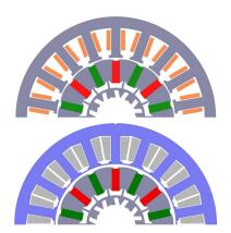
Illustration of a coil arrangement within a pedelec motor with copper coils (top) and an identical motor with cast aluminum coils (bottom). © Fraunhofer IFAM
