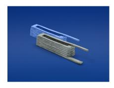
An aluminum coil produced using high-pressure die casting with seven windings and a conductor height of approx. 1.5 mm. © Fraunhofer IFAM
