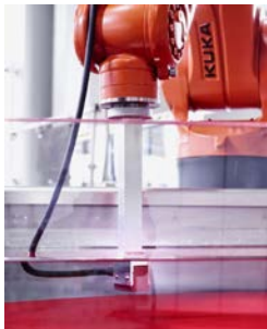
CFRP Ultrasound testing. © Uwe Bellhäuser
