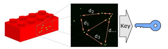
Recognition of individual plastic parts using fluorescent markers. © Fraunhofer IFAM
