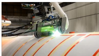
Automated coating of riblets varnish on rotor blades. © Fraunhofer IFAM
