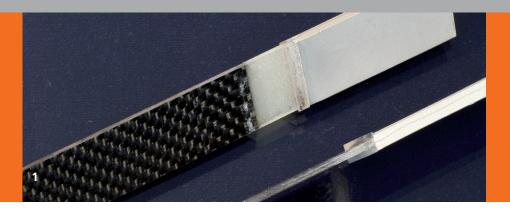
1 CFRP-aluminum hybrid joint.
