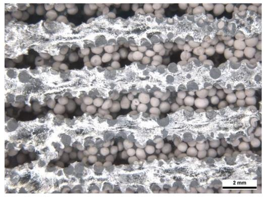
$\Rightarrow$  Very good thermal contact between zeolite and heat exchanger  $\Rightarrow$  Ratio of zeolite/metal and porosity can be adjusted
