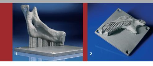
Partial replica of a human jaw bone – laser sintered (with support structure on a building platform).
