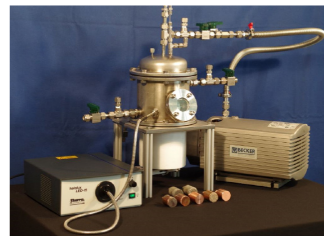
Test rig for evaluating improved heat transfer on structured evaporator surfaces
