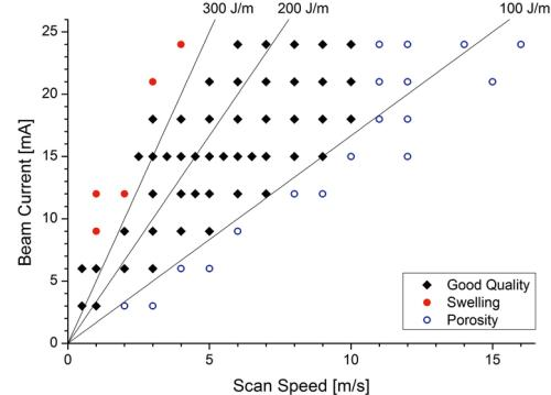
Fig. 1 Processing window for SEBM of Ti-6Al-4V. Blue circles indicate specimens with more than 1 % porosity; red circles indicate pronounced swelling of the surface.
