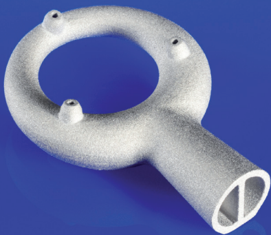
Study of a ring nozzle, status after sintering
