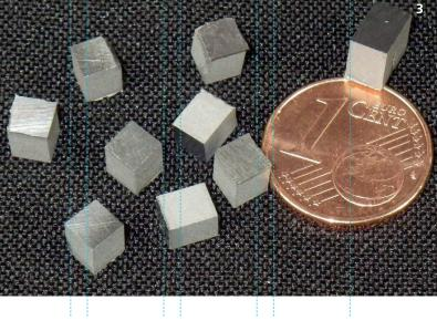
Magnesium- and Manganese-silicides are constituted of inexpensive and low-toxicity elements. They show moderate efficiency (~ 5 %) in a temperature range from 300 °C to 650 °C and the efficiency can still be improved by tailoring the properties via doping.
