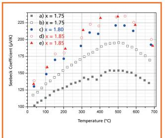
Fig. 2 Seebeck coefficient of MnSi<sub>x</sub> samples with different Silicon content.
