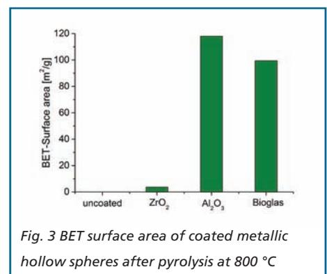
Fig. 3 BET surface area of coated metallic hollow spheres after pyrolysis at 800 °C
