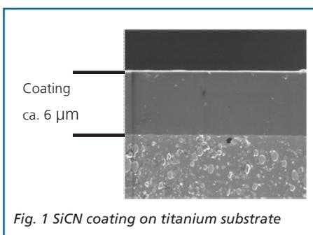
Fig. 1 SiCN coating on titanium substrate
