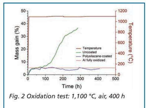
Fig. 2 Oxidation test: 1,100 °C, air, 400 h
